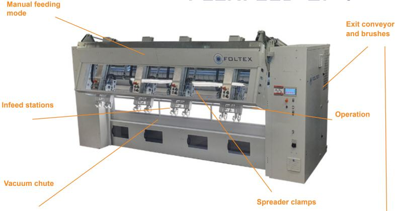
The FLEXFEED LP4 is a versatile feeder for wide range of items like sheets, duvet covers, table cloths, napkins and pillow cases. The FLEXFEED LP4 is provided with 4 infeed stations and is able to work with any ironer. The patented infeed stations lift the item up after feeding and transfers it to servo controlled spreader clamps. After spreading a high power suction beam moves underneath the spreaded item (see picture) for higest feeding quality.
